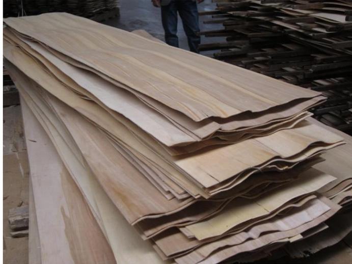
The top veneer might be a thin rotary peeled veneer, or multiple sawn or sliced strips, or a thicker sawn plank between 3mm to 6mm (1/8" to 1/4"). Depending on the factory, they may place face veneers on cut to size cores, one by one. Another option is to place multiple face veneers on a wide core board then cut apart into single planks as shown below:
