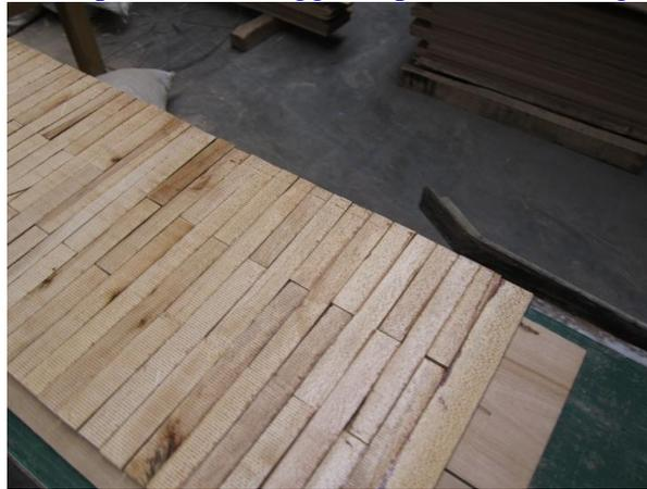
2) Here, the core strips' length equals the width of the final plank. Again there is no glue between the strips. The glue is on the surface of the strips only.
