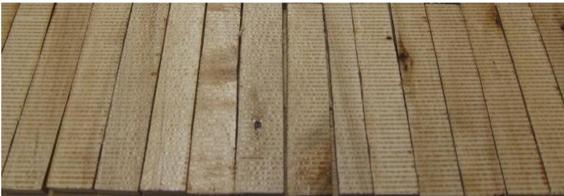
3) In other cases, the small strips are fed into a stringer line where circle saws cut 2 grooves roughly 3mm (1/8”) deep into the surface. String is then pushed into these grooves so the mill can move the core fingers as
