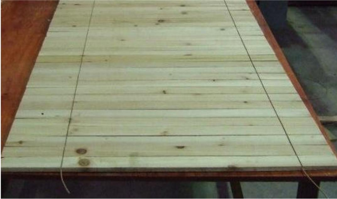
4) Some mills may use a tape (similar to a masking tape) to hold their core strips together prior to veneer gluing, but again, place no glue between the strips.
