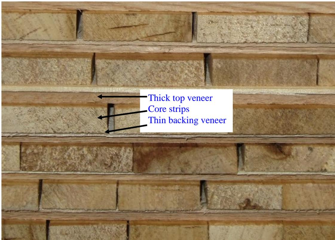
The final floor blank is tongue and grooved. The individual core strips are clearly visible on the tongue.
