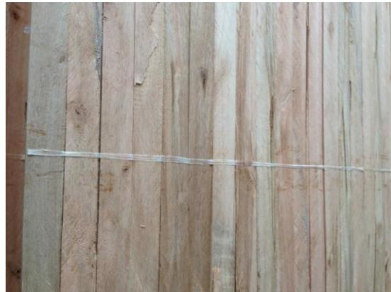
5) Lastly a very few mills will glue the strips together or use an FJL (finger-jointed laminated) core. Here, random width strips are edge-glued together to form the core:
